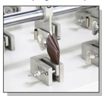
Fixed the end of sample on the upper fixture and fixed the other end on the lower fixture at a angle of 90°.
