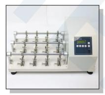
Front view of Bally Resistance Flexing Tester
